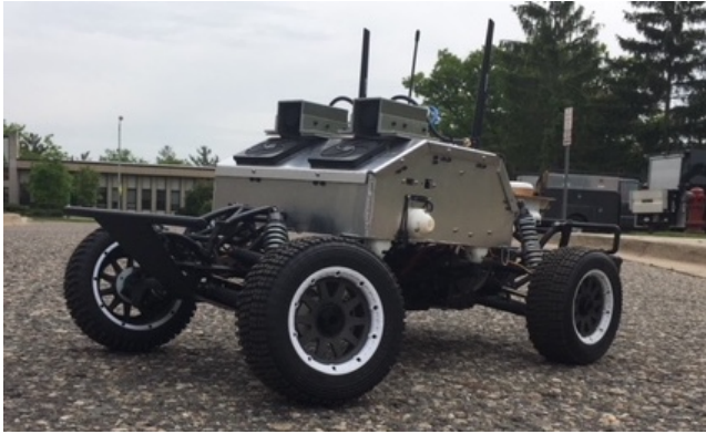
Fig. 1. MSU EvoRally, a 1:5-scale vehicle constructed at Michigan State University, based on AutoRally, an open platform developed by researchers at Georgia Tech [5].
